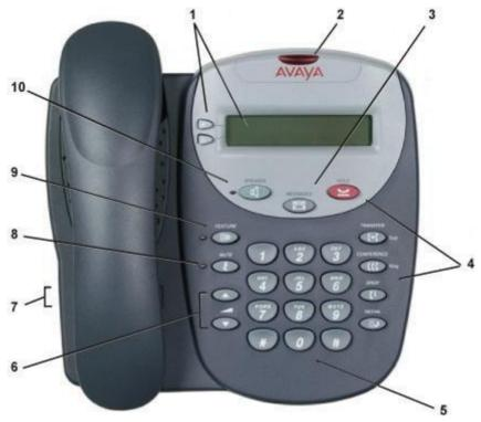
The 2402 display is not fully supported on IP Office. For call appearance icons, caller display etc, the 5402 should be used.
